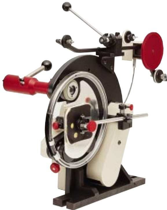
With Slider System Maximum Coil O.D.: 5.0" (127.0 mm) Minimum Coil O.D.: 1.5" (38.0 mm) Minimum Coil I.D.: 0.625" (15.8 mm) Maximum Coil Height: 3.0" (76.2 mm) Wire Size: #22 – #38 AWG (0.64 – 0.1 mm)
